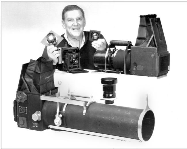
Jim is holding a standard Home Portrait lens in his right hand, and a standard 4x5 R.B. Series D lens in his left hand. To his left is a "Baby Bertha with a 16" f/4.5 Carl Zeiss Tessar, and in front is a Big Bertha with a 40" lens fitted on a Home Portrait. For scale, a 3/4 x 4/4 Speed Graphic is just in front of Jim.
