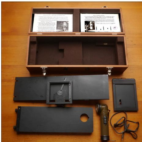
The Graflex Synchronizer Tester<sup>2</sup> is unique among testers in that it is the only one to use gravity as a standard. The testing was done in two phases, the first a visual to get close and the second using flashbulbs and photo paper to get it right on.
