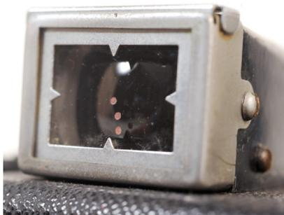
device for centering subjects at very close distances, at 4 feet, 2 feet or 18 inches when the viewfinder rear eyepiece distance is set at 6 feet.
