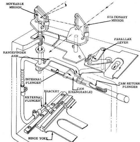
14. The Super has a high-precision built-in rangefinder. The rangefinder cam operates the focusing scale indicator on the stop of the camera, so that the scale always matches the lens used. Shown below is the Pacemaker rangefinder, which is the same system used in the Super Graphic, with a few changes.
