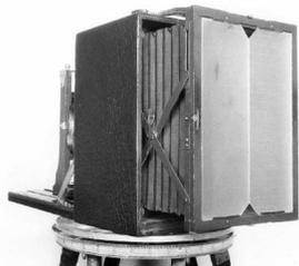
Figure 4. Ground glass in position for focusing, shown folded back in and hinged over prior to film box placed on camera body.
