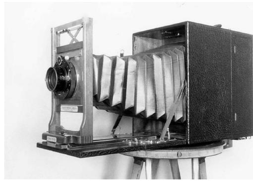
Figure 1. The first No. 10 Cirkut manufactured by Rochester Panorama. Note scissors mechanism to raise or lower the lensboard, which identifies it as an earlier fan type (Model I or II).
