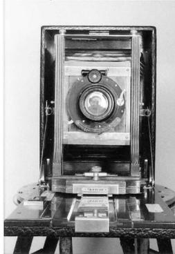
Figure 6. Newly designed lens frame by Locke used on Model III and IV.
