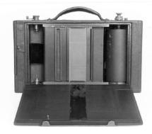
Figure 4. The No. 5 Cirkut with the back open, with the ground glass in position to focus.
