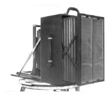
Figure 10. The No. 16 Cirkut with the film box removed with the ground glass extended to focus on the next picture.
