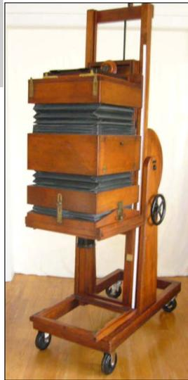
Figure 5. 11"x14" F&S ERC Camera serial number 45416 in vertical position.
