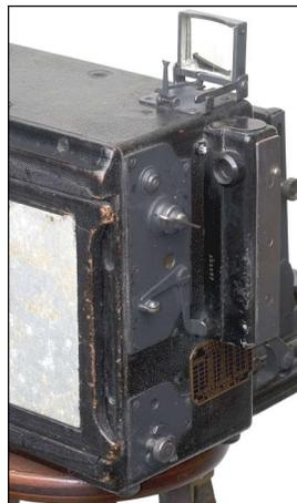
Even more gray painted hardware, and they even replaced/refinished the bed struts! Note the Anniversary style infinity stops and focus scale (coded X14 and designed for a lens of 159.7mm). The bright aluminum focus scale is home-made.
