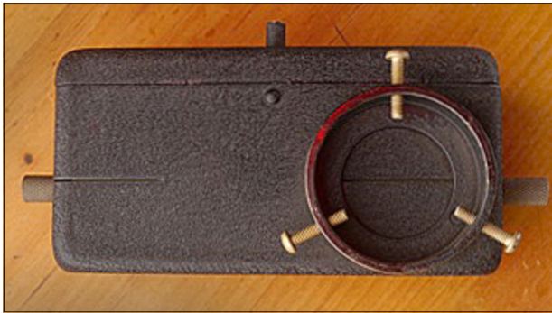
The business end of the tester. The slit on the left is open to record the entire flash. The slit on the right will be restricted by the shutter.
