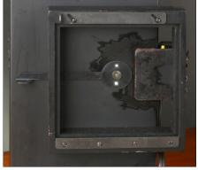
In operation, the lensboard is mounted to the tester. The micro-switch on the right is wired to the trip circuit (behind the red button, on the flash), and the solenoid is wired to the battery case normally. A lever on the tester is set to the center, which opens two small holes behind the lens.
