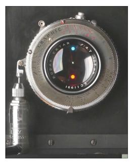
is well, you'll see a blue light at the top, white in the center and red at the bottom. A red light at the top or center means the shutter opened early, a blue light at the center or bottom means the shutter opened late." In operation, colors don't mean a whole lot. If it's not in sync, you won't get three lights. Top, or top and center, means it's early. Bottom, or bottom and center, means it's late.
