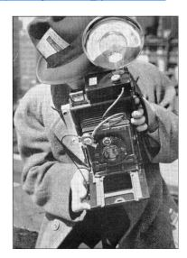
Kalart Micromatic Speed Flash on 4x5 Speed Graphic.
