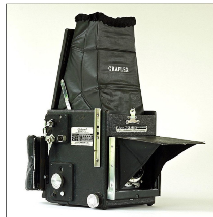
Series D 1/4 plate Graflex. Also in 4x5, its focal plane shutter gave a choice of 25 speeds to 1/1000 plus T.
