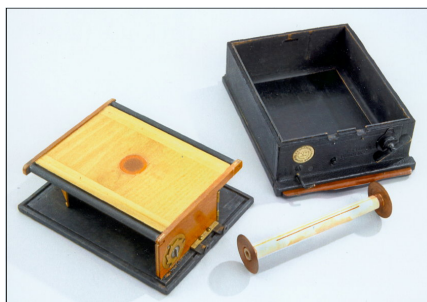
Disassembled roll film holder from case at top left.
