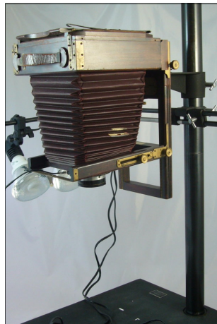
Left, Photorecord stand in use with 4x5 Graphic View Camera, and right, stand with a 5x7 Eastman Medical Camera.
