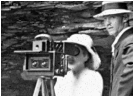
Early glass slide showing Triple Lens with taking lenses diaphragms linked with an aperture bar, similar to that used on a Stereo Auto Graflex.
