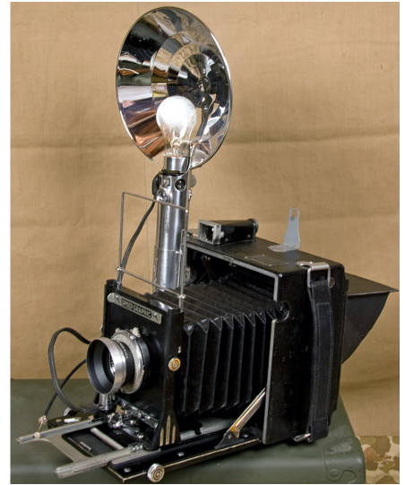
Figure 5: Army Air Force contract camera viewed from the right side. Overall a nice pre-war example of a black leather-covered body and lots of the classic chrome trim. This Speed Graphic is fitted with a Kodak Ektar 127mm lens. The lens has a Kodak Series VI lens shade affixed, and the lens is mounted in a Kodak No. 2 Supermatic shutter, tripped by a No. 2 Kodak solenoid attached by electric cable direct to the Graflex flash mounting a 7" reflector. There is a Graphic back, and the rear viewing door is visible in the open position – set up for ground glass focusing. (Author's Collection)
