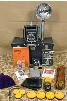
Figure 3: A closeup of my reconstruction of Theo Hios' camera, based on photos of him with his camera: Graflex 3 cell flash mounting a 5" reflector which mounts on the exterior of the Kalart Synchronized Rangefinder. The camera is an all-black wartime model, serial number 337346, probably made around 1943-1944. The lensboard slide bar does not bear the “Speed Graphic” logo. The black wood “C” board is fitted with a No. 2 Supermatic shutter with a Kodak Ektar lens, serial number EA4061. “EA” is the Kodak code for 1942. The solenoid mounted to the left of the lens is a Graflex #3. The back is the 4x5 spring-loaded Graphic back which can take the 12 shot film packs or 2 sided plates. (Author's Collection)
