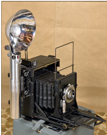
Figure 2: A recreation of Sgt. Theo Hios' Speed Graphic camera. Based on evidence presented in my previous article, I was able to reconstruct this facsimile of the Anniversary Speed Graphic issued to Sgt. Hios, ca. 1943. The camera has all the correct features – 4x5 Format, 127mm Ektar lens in a Kodak No. 3 Supermatic shutter on a wood “C” lensboard. Wartime manufactured cameras also made less use of chrome plated parts, as this one is mostly black, except for the lens/shutter and Kalart rangefinder. A Graflex solenoid is mounted to the left of the shutter. Although obscured by the 5" reflector on the Graflex flash, the data plate on this camera is located to the left side bottom, near the rear shutter cocking knob. Just to the right of the camera is a Weston Master Model 715 Universal Exposure Meter. The tan canvas musette bag is actually an original piece of equipment issued to Theo Hios (His name, rank and unit number are all stenciled on it.). This was the carryall bag that he took in all the invasions with the 4 th Marines in the Pacific (Roi-Namur, Saipan-Tinian and Iwo Jima). In addition to hauling his Speed Graphic, he also carried his artist sketch pads, brushes, pens, paints, etc. To the extreme left is his original steel pot helmet, and the knife near the center is his “Ka-Bar” USMC issue combat knife. (Author's Collection)
