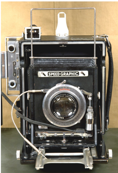
Figure 5: Army Air Force contract camera viewed from the right side. Overall a nice pre-war example of a black leather-covered body and lots of the classic chrome trim. This Speed Graphic is fitted with a Kodak Ektar 127mm lens. The lens has a Kodak Series VI lens shade affixed, and the lens is mounted in a Kodak No. 2 Supermatic shutter, tripped by a No. 2 Kodak solenoid attached by electric cable direct to the Graflex flash mounting a 7" reflector. There is a Graphic back, and the rear viewing door is visible in the open position – set up for ground glass focusing. (Author's Collection)
