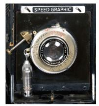
ter. A closeup view of the lens itself tells of its origin: a Wollensak 127mm Velostigmat lens, being a contender for the more commonly observed Ektar lens made by Kodak (author's collection).
