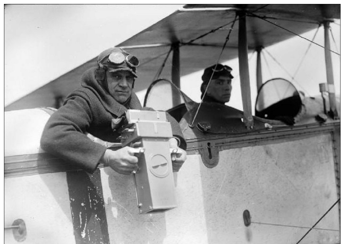
Albert Stone sits in rear of biplane (ca. 1919) holding an early version of the Graflex Aero Camera, Model A-1.
