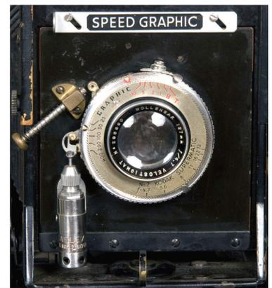
A closeup view of the lens itself tells of its origin: a Wollensak 127mm Velostigmat lens, being a contender for the more commonly observed Ektar lens made by Kodak (author’s collection).
