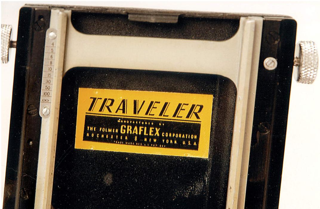
This illustration should have been included with the following text from Jim Chasse's article: "What does set it apart from the Miniature, other than the lack of a focal plane shutter, is the yellow and black decal in the well and the plastic pieces attaching the focusing rails."
